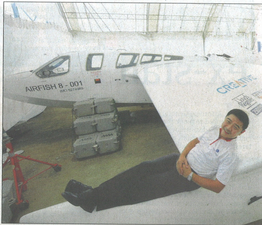
Wigetworks general manager Kenneth Tan, with the AirFish 8, which can cruise 6m in the air over a mass of water, on an air cushion produced by aerodynamics. ST PHOTO: AZIZ HUSSIN
